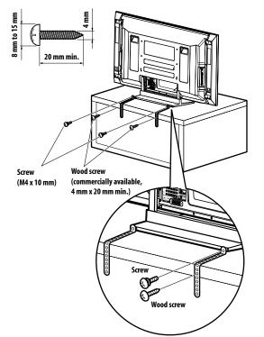
Drill a hole in the middle at the rear of the tabletop panel before using a wood screw. Perform this work the same way on the left and right sides.
